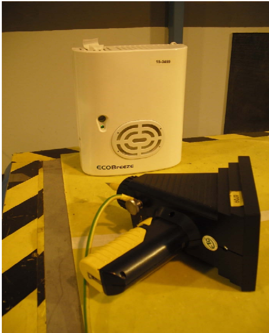
Photograph 3: Electrostatic Discharge Setup
