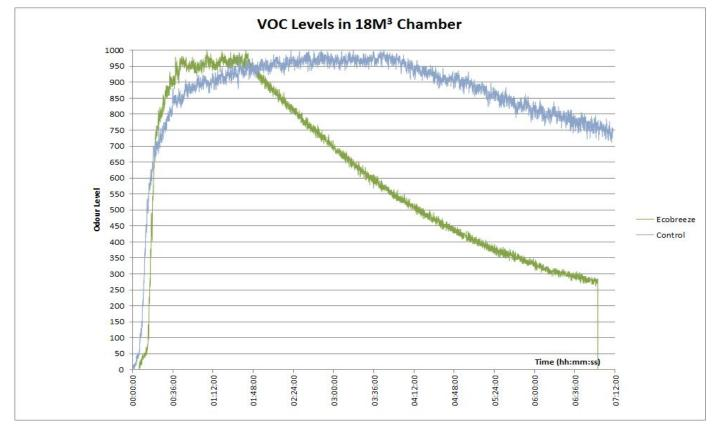
This chart clearly demonstrates the performance of the **ECOBreeze unit** in reducing VOC levels and consequently odour levels in an 18m<sup>3</sup> chamber over a 7 hour period as against a control.
